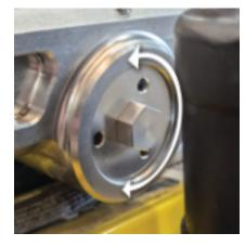
Lightly tighten one of the M6 Grub Screws and test the mesh by turning the steering wheel left and right. The goal is to find a balance between a notchy steering feel and rotational play in the steering rack.
