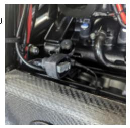
Locate and disconnect the Suzuki K-Line to AIM Dash connector at the back, left hand side of the engine as shown.
