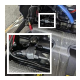
Unplug the connector and insert it into the back of the standard instrument cluster. This will display possible fault codes once the ECU is put into code display mode.
