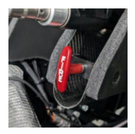
There is an additional pull-ringon top of the air box under the main roll hoop for marshals to activate the system from outside the car.
