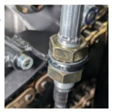
The ratio can be adjusted with the 2 positions on the gear lever. The top hole will give a lighter shift with a longer throw. The bottom hole will give a heavier shift with a shorter throw.
