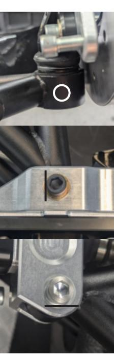
Use a digital angle gauge to ensure that the castor on both sides are equal. It is OK to deviate from these measurements in order to make the castor even on both sides.
