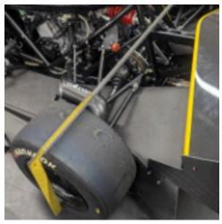
Make sure that the speed square is sitting flat against the straight edge, and that the speed square is just touching the outside of the tyre.
