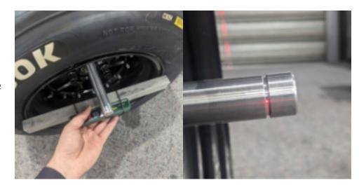
Alignment with the grooves on the toe adjustment pins will achieve 0.5 degrees of toe in for both front and rear wheels.
