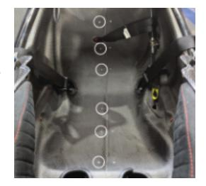
When removing the seat, you will first need to remove all of the M6 chassis screws around the perimeter of the seat, to relieve any tension, then you can remove the left M5 BHCS screws before removing the left seat shell. You cannot remove the RIGHT seat shell before removing the LEFT seat shell.
