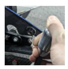
When slowly releasing the clutch, you may find that the car does not move, or you may find that the car wants to roll forward. If the car tries to roll forwards, turn the adjustment screw located on the clutch slave cylinder clockwise until you can release the clutch and the car does not move.
