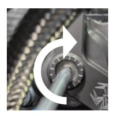
**Counterclockwise**will bring the clutch plates together and lower the slip adjustment.
