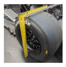
A measurement of 17mm will equate to 2.5 degrees of negative camber which is the factory setting. For your own reference, 21mm will equate to 3 degrees and 14mm is 2 degrees.
