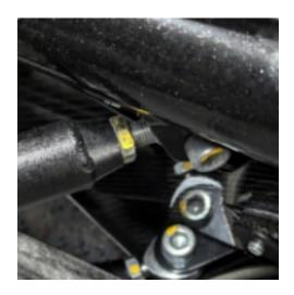
**NOTE:** Adjusting these rod ends to set caster will also alter the camber adjustment, this will either need to be taken into consideration when making caster adjustments so that camber is not changed, or you can adjust the camber shims to adjust this independently.
