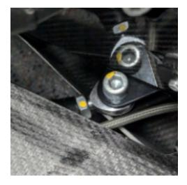
Or, by moving the upper portion of the upright backward or forward using the rod end at the back of the upper control arm.
