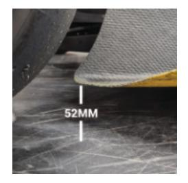
Set the rear tunnel height by measuring and 60mm between the ground and the underside of the tunnel as shown.
