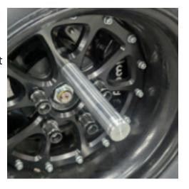
Hold the laser alignment tool up against the wheel you wish to set the toe, and adjust it using the appropriate adjustment rod until the laser aligns with the groove on the opposite alignment pin.
