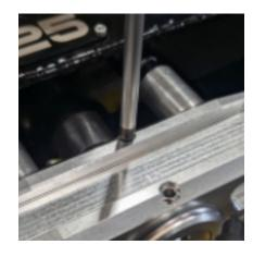
Turn the front mesh adjuster in either direction until it begins to tighten.
