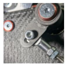
The gear cable does not require any maintenance, however, excessive force at the shift lever can cause the cable to snap. It is recommended to carry a spare and replace this cable once per year.
