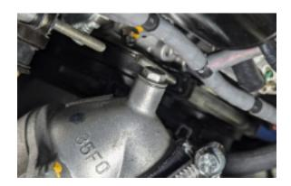
Locate the crossover radiator hose that sits in front of the engine, this is fitted with a bleed fitting on the left-hand side just behind the fuel filler neck.
