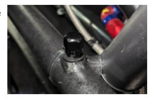
Filling is recommended to be completed with 2 people, where one person can fill and the other can remove and install bleed screws around the car.
