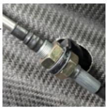
If you have run out of adjustment in the cockpit, the same adjustment can be performed at the other end of push/pull cable in the engine compartment.
