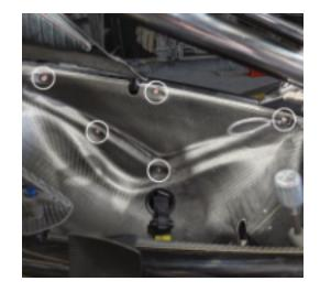
**WARNING:** The left portion of the joining strip has integrated nut plates to allow for the M5 BHCS screws to be removed and installed without needing to access the back of the seat halves. The right-hand side of the joining strip is bolted directly to the right-hand seat half with Nyloc nuts, and should not be removed. The joining strip will remain bolted to the right-hand seat half.
