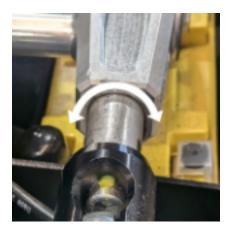
**IMPORTANT:**It is OK to feel a small amount of stiffness or notching in the steering when trying to mitigate the rotational play in the rack, this will not be felt when the car is on the ground.
